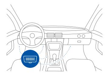
Most common OBDII connector locations.
